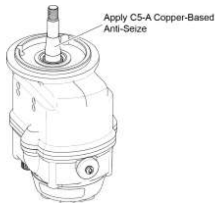
Figure 3 C5-A Copper-Based Anti-Seize Application
