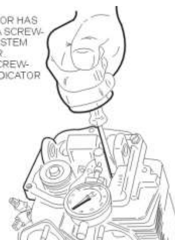
Figure 9 Pushing Valve Stem and Adapter Post Toward Dial Indicator
