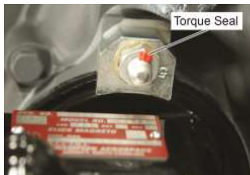
Figure 5A Torque Seal on the Magneto Nuts
