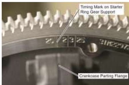
Figure 1 Timing Marks on the Crankcase Side of the Starter Ring Gear Support Assembly Aligned with the Crankcase Parting Flange
