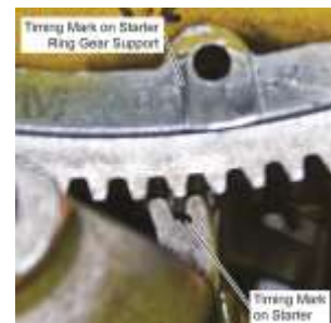
Figure 2 Timing Marks on the Propeller Side of the Starter Ring Gear Support Assembly Aligned with the Timing Mark on the Starter
