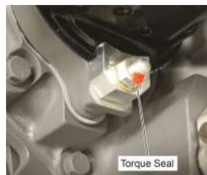
Figure 5A Torque Seal on the Magneto Nuts
